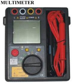
**APPLICATION :** Measurement of the Insulating resistance of various insulating materials and electric equipments such as Transformer, Motors, Cables, switches and electric apparatus. Also applicable to maintenance, test and inspection of various electric equipments.
