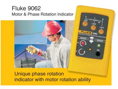
The Fluke 9062 Motor and Phase Rotation Indicator is a portable, handheld instrument designed to detect the rotary field of three-phase systems and motor direction. And without hooking up test leads, you can determine the rotation of a motor by holding the tester above the motor in line with the shaft. Like other tools that you have come to expect from Fluke, the 9062 is rugged, reliable, and easy to use. If you frequently work on motors, this tester is a must have for your tool belt.
